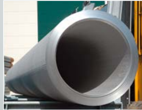
Plates are edged or formed and then welded into pipes
